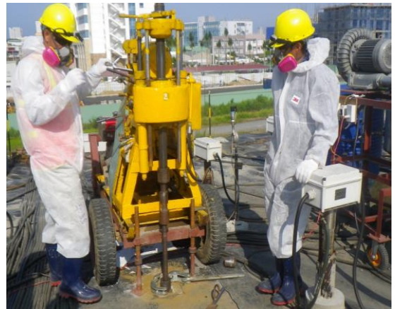
Phase 2 post-treatment confirmation sampling on top of the treatment structure. (Photo: CDM Smith)
