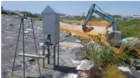
Collecting ambient air samples from the perimeter of all earthworking activities (Photo: CDM Smith)
