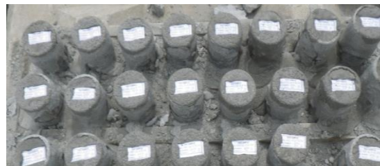
Samples of lightweight insulating concrete for strength and other physical property testing (Photo: CDM Smith)
