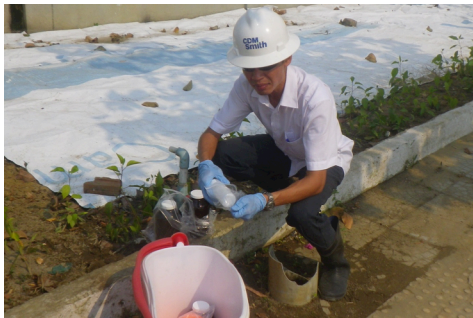
Collecting a groundwater sample from an offsite well (Photo: CDM Smith)
