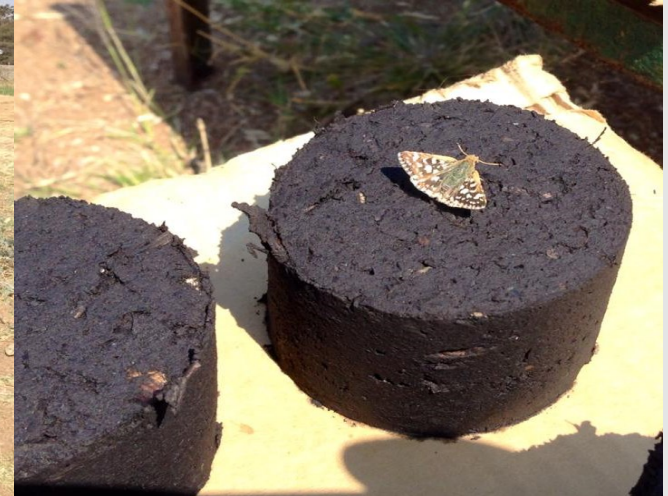
August 2014: Steve Collins, RESILIM Biodiversity Activities Manager, and the Botswana Department of Water Affairs successfully test the production of charcoal briquettes from dried water hyacinth
