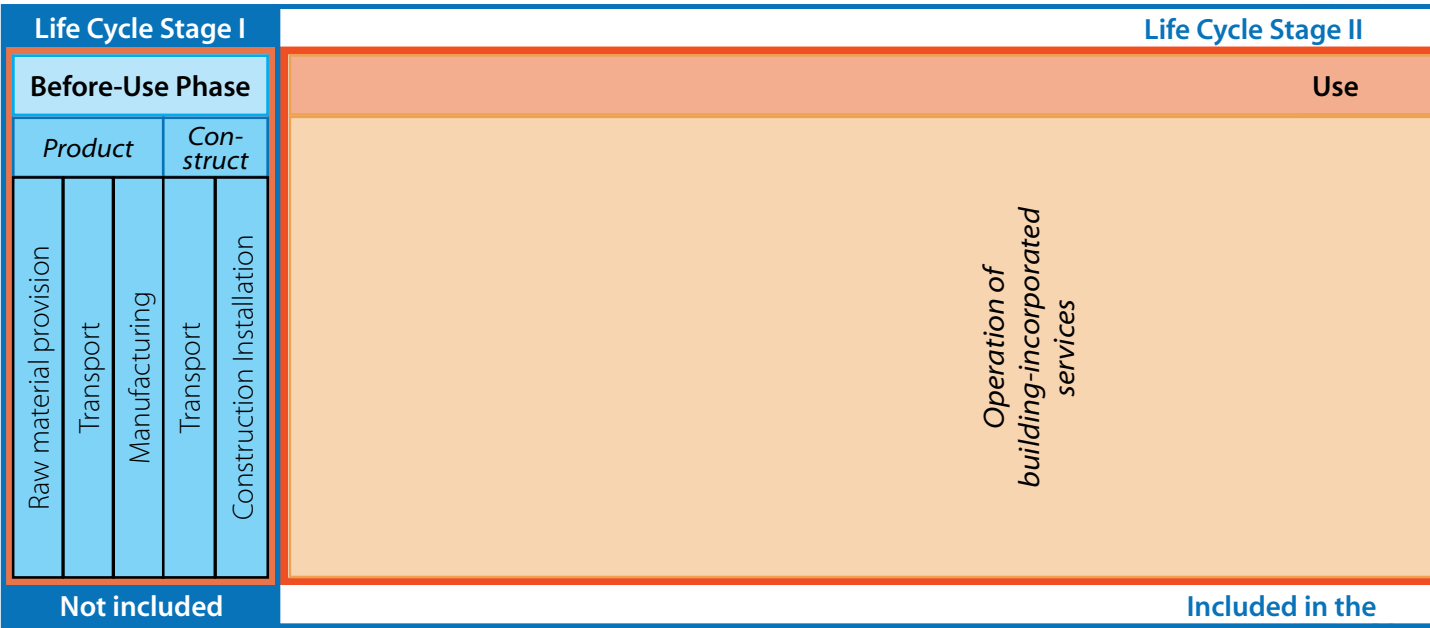
Figure 2: Description of the three Life Cycle Stages of a building and the different processes allocated to these stages, (Source: SB Alliance)
