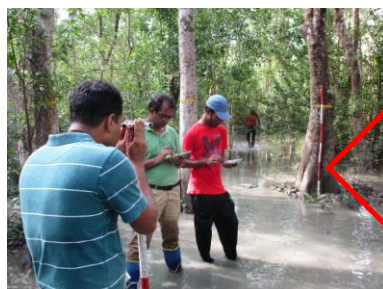
Figure 23: Bearing measurement using Suunto clinometer
