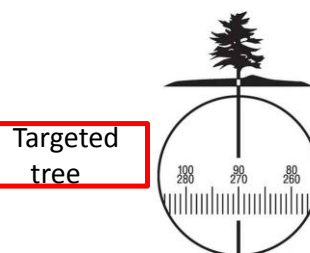
Figure 23: Bearing measurement using Suunto clinometer
