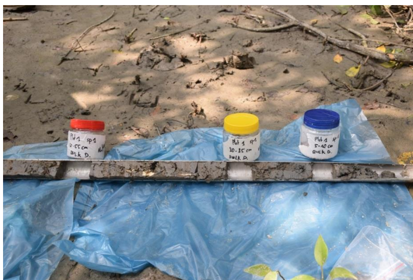
Figure 34: Bulk density cores are extracted from the long auger in the Sundarbans. Use a tape measure to extract exactly 5cm length sections at intervals between 0-15, 15-30, and 30-100.
