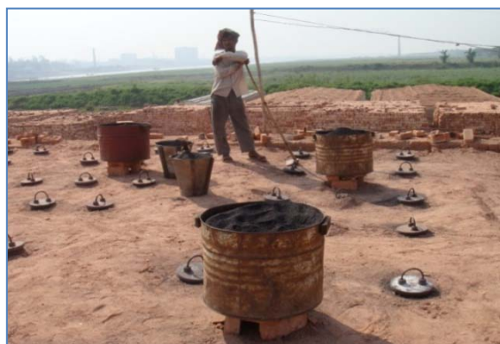
Figure 3.5 Firing bricks. There are 18 furnaces on top of each chamber through which coal is poured intermittently for burning the bricks.
