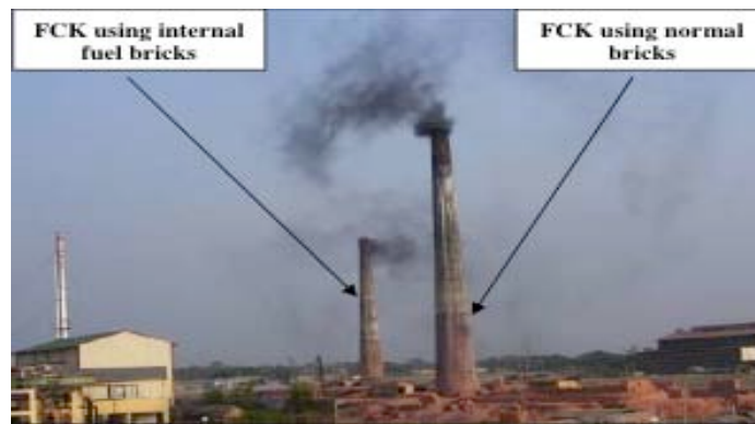
Figure 4.1: Comparison of FCK and IFCK emission reductions
