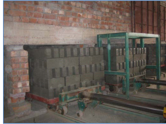
Figure 3.8 Mechanical transport of green bricks.
