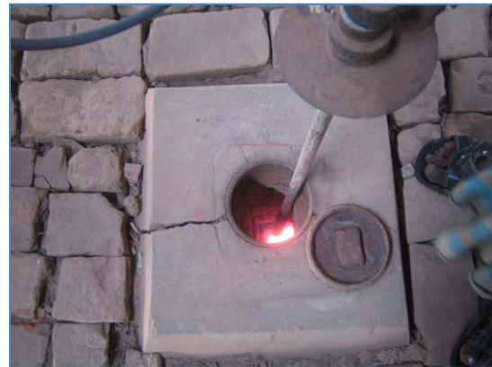
Figure 3.10 Gas pipeline to the brick chamber for firing bricks.
