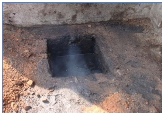
Figure 3.4 Deposited residues from smoke. Smoke from the chamber comes to a channel before it is released. The channel is connected to another underground channel which is half filled with water. The smoke and vapor from the kiln is extracted by a blower pump. Since the smoke flows over water into the underground channel, a large portion of the suspended particulate matter is extracted from the smoke and deposited.
