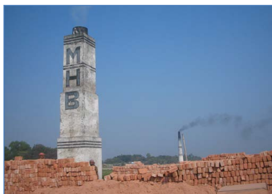
Figure 3.6 In the front the zigzag chimney emitting cleaner smoke, than the FCK black smoke in the rear.
