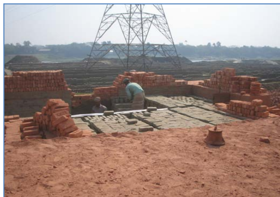
Figure 3.1 31 Placing bricks for firing: Bricks are placed in blocks in each chamber according to the shape and size of the chamber. In this picture, each block has 7 columns, each column contains 13-18 bricks, and there are 17-21 layers of brick.
