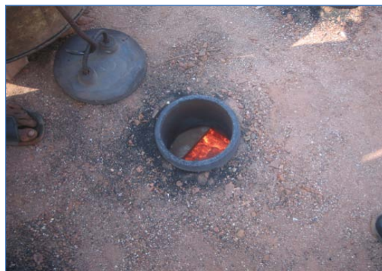
Figure 3.2 One of the furnaces on top of a chamber through which coals are poured.
