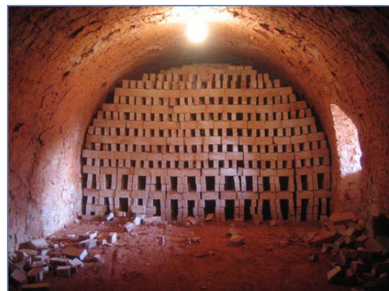
Figure 3.12 Outlet for burnt brick collection.
