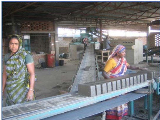
Figure 3.11 Semi mechanically molded green bricks.
